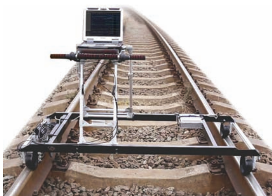
Fig. 6. Defectoscope for single rail inspection [17]
