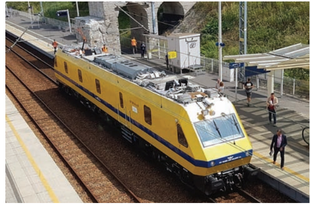
Fig. 5. Railway measurement trolley [3]
