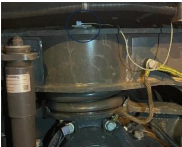
Fig. 9. Measurement point 1 localized on the train bogie [photo: A. Łomżyńska]
