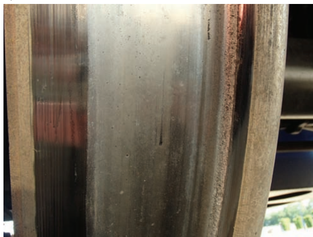
Fig. 17. (a) Rolling surface of a wheel with a cast iron insert ( R_a = 2,11\mu\text{m} ), (b) surface of a wheel with a K-type composite insert ( R_a = 0,47\mu\text{m} ) [photo: P. Tokaj]
