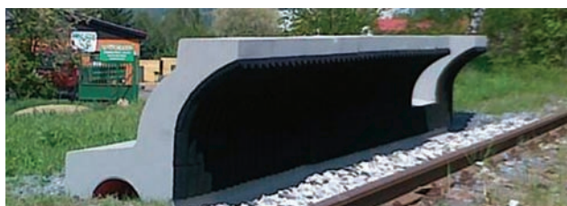
Fig. 18. Low noise barrier to protect against the rolling noise [source: UIC]
