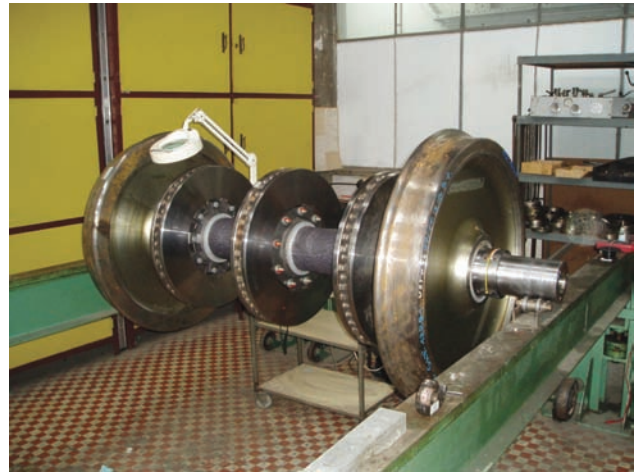
Fig. 3. Wheelset during installation preparation for QY force measurement [photo: A. Zbieć]
