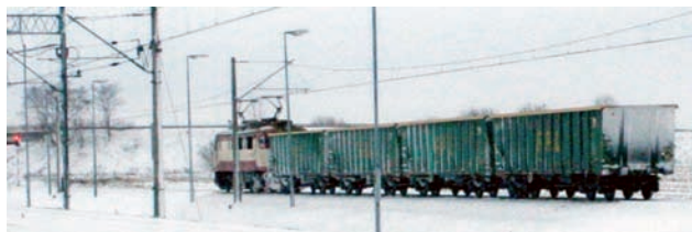
Fig. 16. Composition of a train for the noise study conducted at the Institute's experimental track in Żmigród [photo: P. Tokaj]
