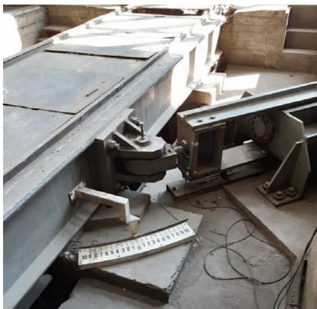
Fig. 15. The Railway Research Institute's test stand for measuring the moment of resistance of bogies relative to the body [photo: A. Chojnacki]
