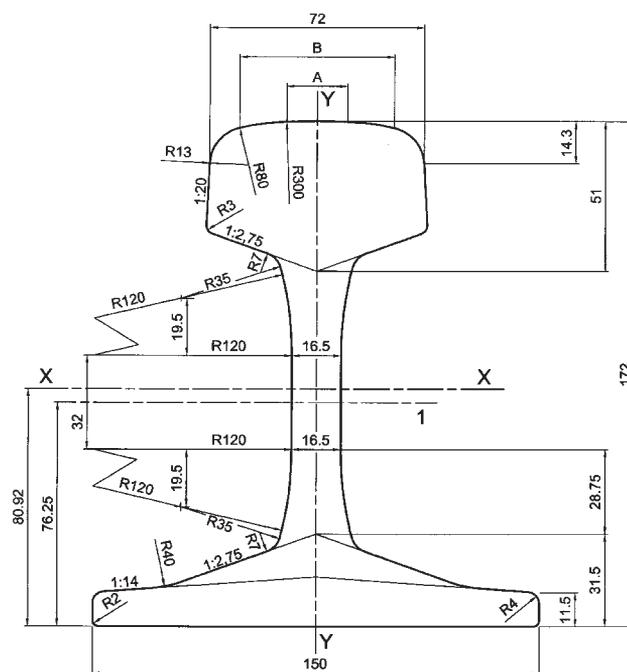
Fig. 2. Vignoles rail with a 60E1 profile; dimensions in millimetres [31]
