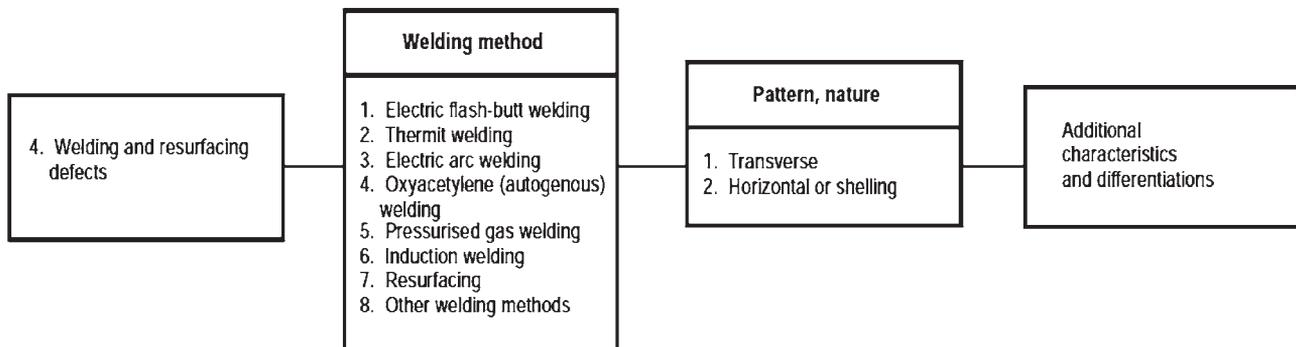
Fig. 3. Diagram of rail joint defects; author's own elaboration based on [32]
