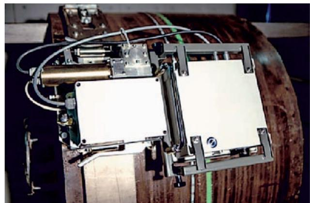
Fig. 6. Scanner together with a DR detector guided on a Cross tape during the testing of peripheral joints [50]
