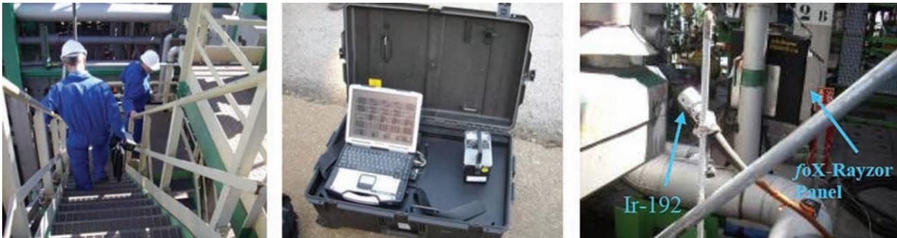
Fig. 5. Work in a refinery with a portable Digital Radiography (DR) system [45]
