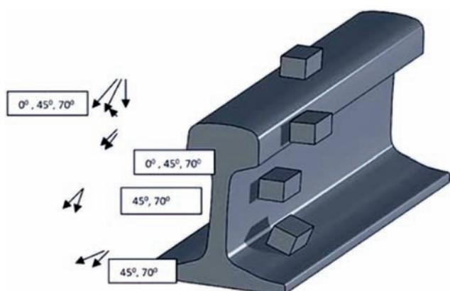
Fig. 1. Probe positioning during UT testing of rails [30]
