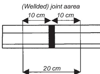
Fig. 4. Rail joint area [35]
