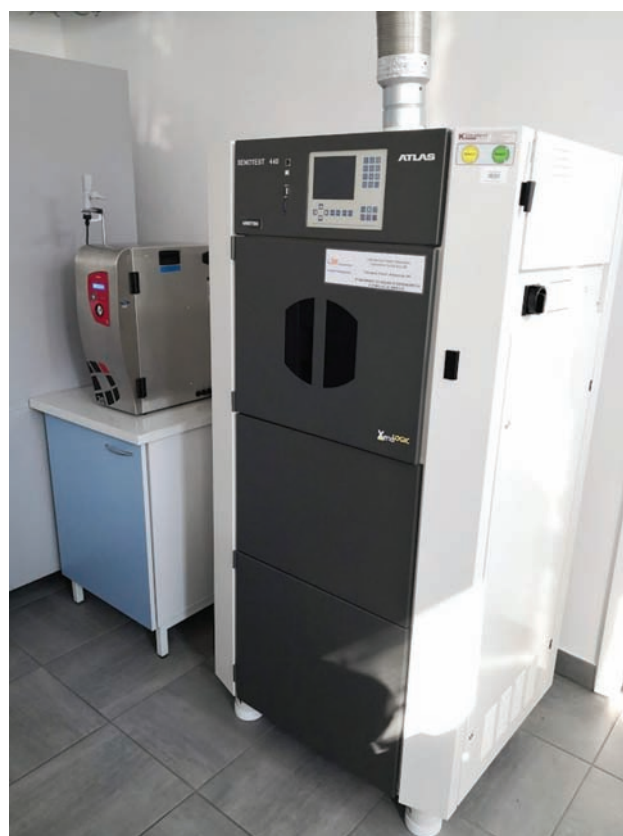
Fig. 1. Test stand for ageing samples according to ISO 16474-2 [7] (xenon weathering instrument, Atlas GmbH Xenotest 440) [Pic. M. Garbacz]
