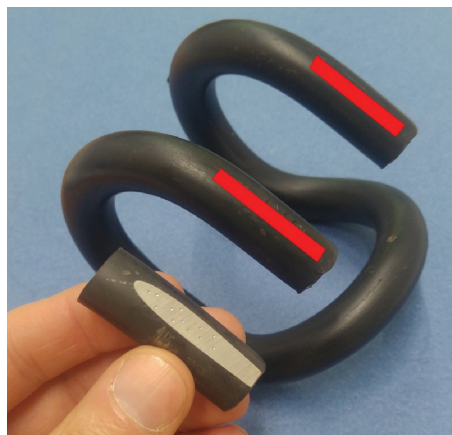
Fig. 3. An SB4 spring clip with the hardness measurement place marked in red and a ready sample with post-hardness testing traces [photograph by A. Aniszewicz]
