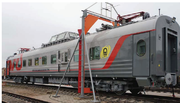
Fig. 5. The Integral car on the measuring instrument calibration station [19]
