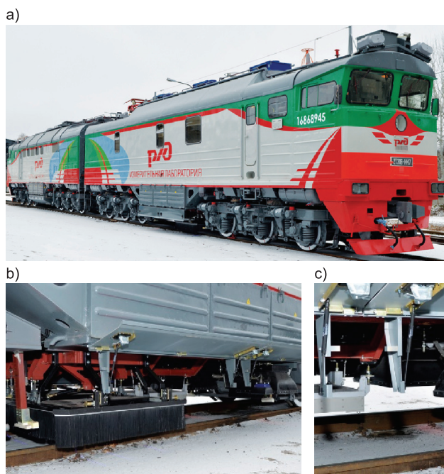
Fig. 10. SMDL- 2TE116 measuring diesel locomotive [6]; a) View of the locomotive, b) Rail condition laser monitoring devices, c) GPR for monitoring the substructure, d) Overhead contact line condition monitoring equipment
