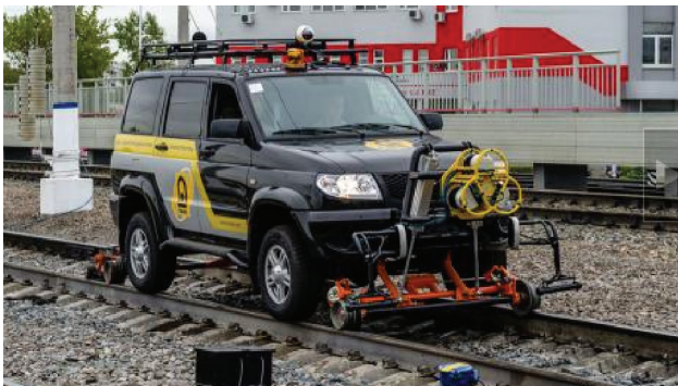
Fig. 14. Road vehicle used for trackside infrastructure measurements [12]
