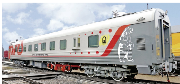
Fig. 6. The VD-UMT-2 flaw detector car is designed for complex diagnostics of railway infrastructure using ultrasonic, magnetic and optical non-destructive testing methods [17]
