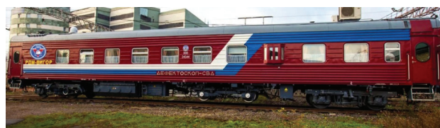
Fig. 3. RDM – WIGOR flaw detector car [14]
