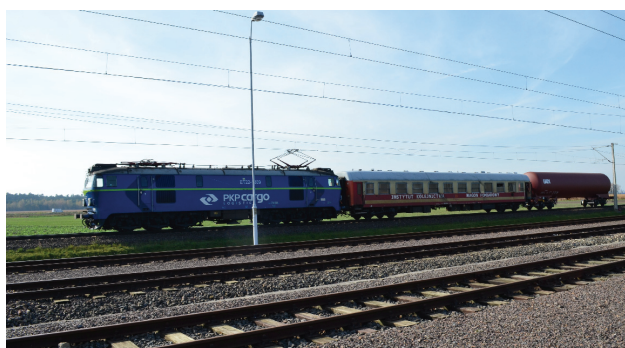
Fig. 6. Measuring train set for testing the braking system of the tank car [own elaboration]
