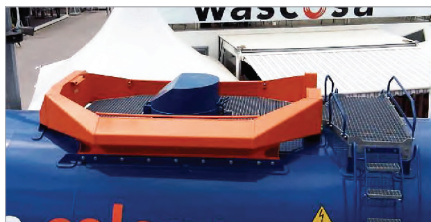
Fig. 7. A UE01 module protecting tank filling valves in the event of tipping over [1]
