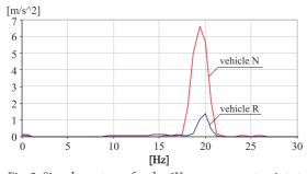
Fig. 3. Signal spectrum for the 6Y measurement point at 40 km/h; main components: vehicle N – 19.38 Hz, 6.6 m/s<sup>2</sup>, vehicle R – 20.00 Hz, 1.4 m/s<sup>2</sup> [own study]
