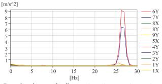
Fig. 5. Signal spectra for all measuring points on an inoperative vehicle at a speed of 70 km/h [own study]
