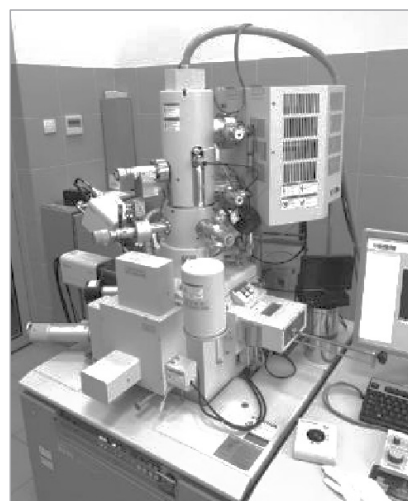
Fig. 2. Scanning electron microscope used for the research – HITACHI SU-70 [photo. K. Franczak]
