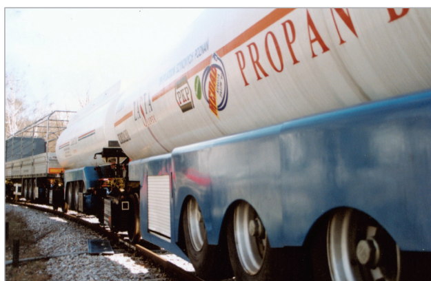
Fig. 17. Bimodal unit in a railway composition [photo. A. Zbieć]
