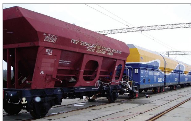
Fig. 19. Four-section short-coupled self-discharging wagon with two-axle sections photo. A. Zbieć]
