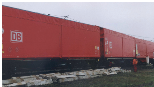
Fig. 20. Two-axle wagon with sliding walls tested in the additional variant in which the wagon is surrounded by two identical wagons [photo. A. Zbieć]
