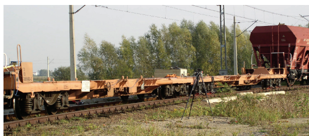
Fig. 21. Two-section platform wagon on four bogies [photo. A. Zbieć]
