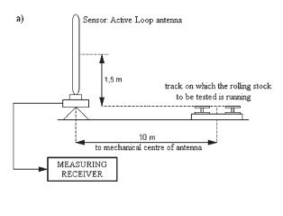
Fig. 1. Antennas required for measuring radiated disturbance emission: a) active rectangular magnetic loop antenna, b) biconical dipole, c) log-periodic antenna [The authors' own figure]
