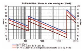
Fig. 3. Permissible levels of radiated disturbance emission for railway rolling stock during the drive [The author's own figure]
