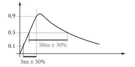
Fig. 5. The graph BURST 5/50 ns impulses [Own figure]
