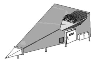
Fig. 2. The GTEM chamber [Own figure]
