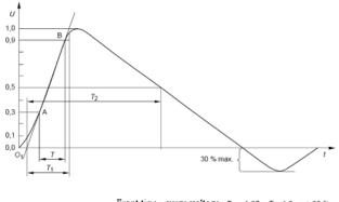
Front time - surge voltage:  $T_1 = 1,67 \times T = 1,2 \ \mu s \pm 30 \ \%$ Multicycle time  $T_2 = 50 \ \mu s \pm 20 \ \%$ .
