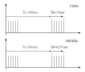
Fig. 6. BURST of disturbance impulse parameters for f = 5 kHz and 100 kHz [Own figure]
